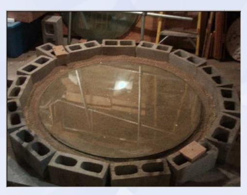
60 inch disk of glass on it's mold. It took two men and a third for positioning to put in in place. It was dropped taking it out.
